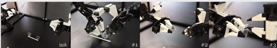
Open Cup: Pick up and open the lid of a translucent condiment cup. The cup is randomized along the 15cm white line. Both arms approach the cup, and the right gripper gently tips over the cup ( Subtask#1 Tip Over ) and pushes it into the gripper of the left arm. The left arm then gently closes its gripper and lifts the cup off the table ( Subtask#2 Grasp ). Next, the right gripper approaches the cup lid from below and prys open the lid.
