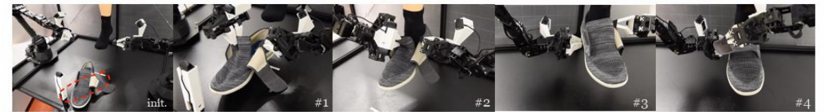
Put On Shoe: Put a velcro-strap shoe on a fixed mannequin foot. The shoe pose is randomized along the 15cm white line. First, both left and right grippers pick up the shoe ( Subtask#1 Lift ). Then both arms coordinate to put it on, with the heel touching the heel counter ( Subtask#2 Insert ). Next, the left arm moves to support the shoe ( Subtask#3 Support ), followed by the right arm securing the velcro strap ( Subtask#4 Secure ).
