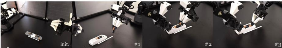
Slot Battery: Insert the battery into the remote controller. The controller is randomized along the 15cm white line. The battery is initialized in roughly the same position with different rotations. The right arm first grasps the battery ( Subtask#1 Grasp ) then places it into the slot ( Subtask#2 Place ). The left arm presses onto the remote to prevent it from sliding, while the right arm pushes in the battery ( Subtask#3 Insert ).
