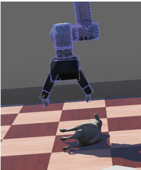
Fig. 18. Errors occur when there is a mismatch in size between the fixture and the object being grasped.
