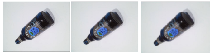
Fig. 6: a) Original b)Max pooling with 3*3 c) Max pooling with 5*5
