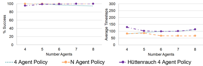
Fig. 7. The success rate and average timesteps on the repulsive evader benchmark, comparing our full approach (trained on the appropriate amount of agents), the approach by Hüttenrauch [6] which was trained on four agents and our approach which was limited to only see the closest four agents during execution.
